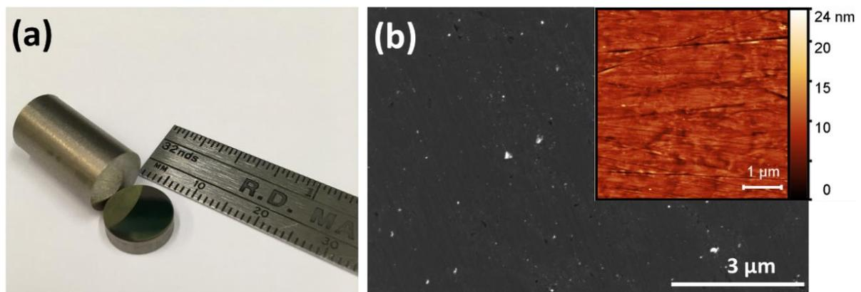
**Figure 1.** (a) Photograph of the targets used in this work: 3-mm height disks from 1-cm diameter titanium bars were cut and mechanically polished. (b) SEM image of the initial surface morphology of *as-polished* titanium samples before ion irradiation and AFM micrograph (inset). In this way, *as-polished* samples can be produced with a surface roughness below  $\sim 2$  nm.
