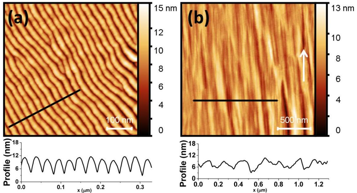
**Figure 3.** AFM micrographs of Ti targets after  $\text{Xe}^+$  irradiation at  $\alpha =$  (a)  $0^\circ$  ( $\lambda = 28$  nm,  $R_q = 2.25$  nm) and (b)  $80^\circ$  ( $\lambda = 180$  nm,  $R_q = 1.43$  nm). For  $\alpha = 80^\circ$ , the arrow indicates the ion beam projection on the surface. One-dimensional profiles are given underneath the topography images.
