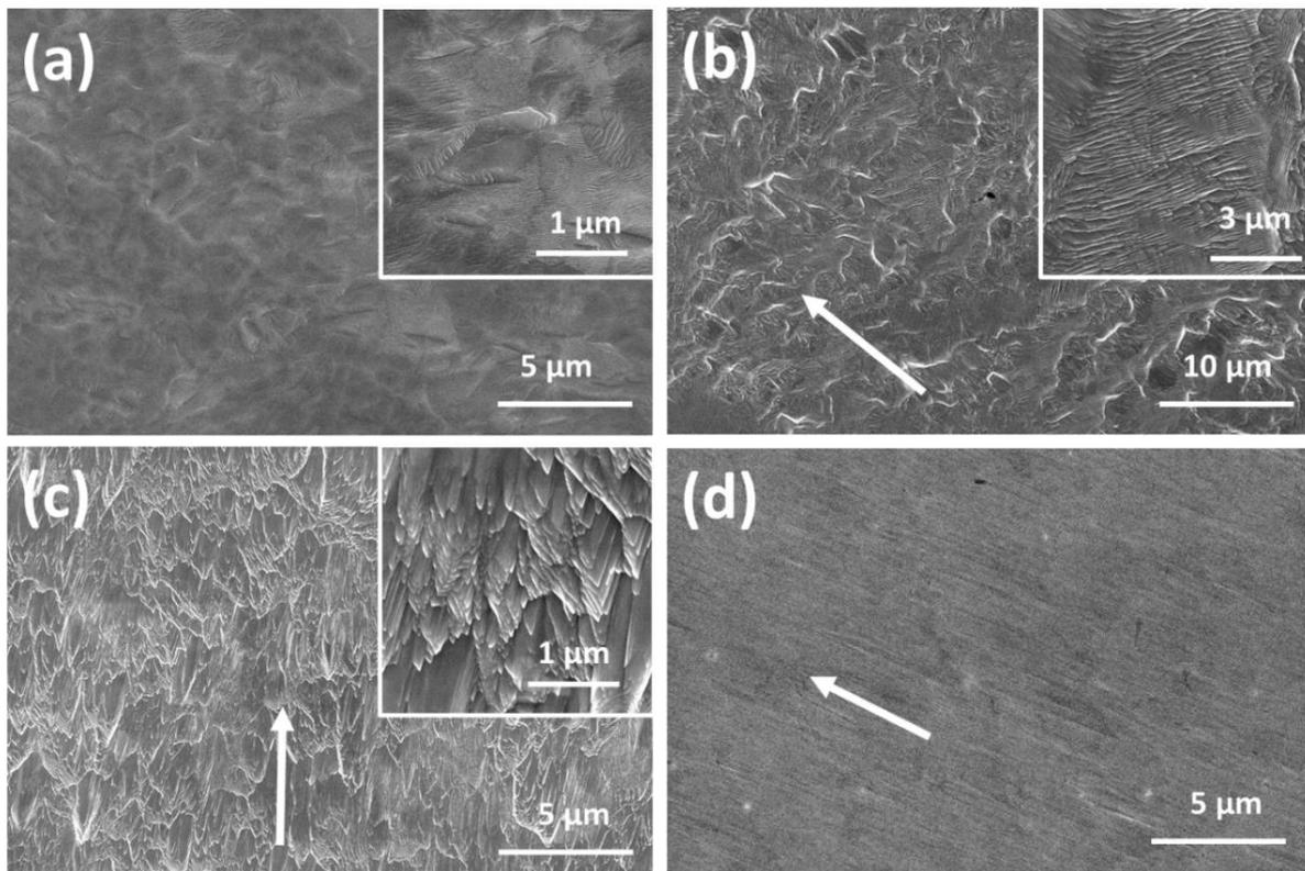
**Figure 2.** SEM micrographs of titanium irradiated surfaces at  $\alpha =$  (a)  $0^\circ$ , (b)  $60^\circ$ , (c)  $70^\circ$  and (d)  $80^\circ$ . When shown, the arrow indicates the projected ion beam direction onto the surface. The insets are images of the surface features with a higher magnification.
